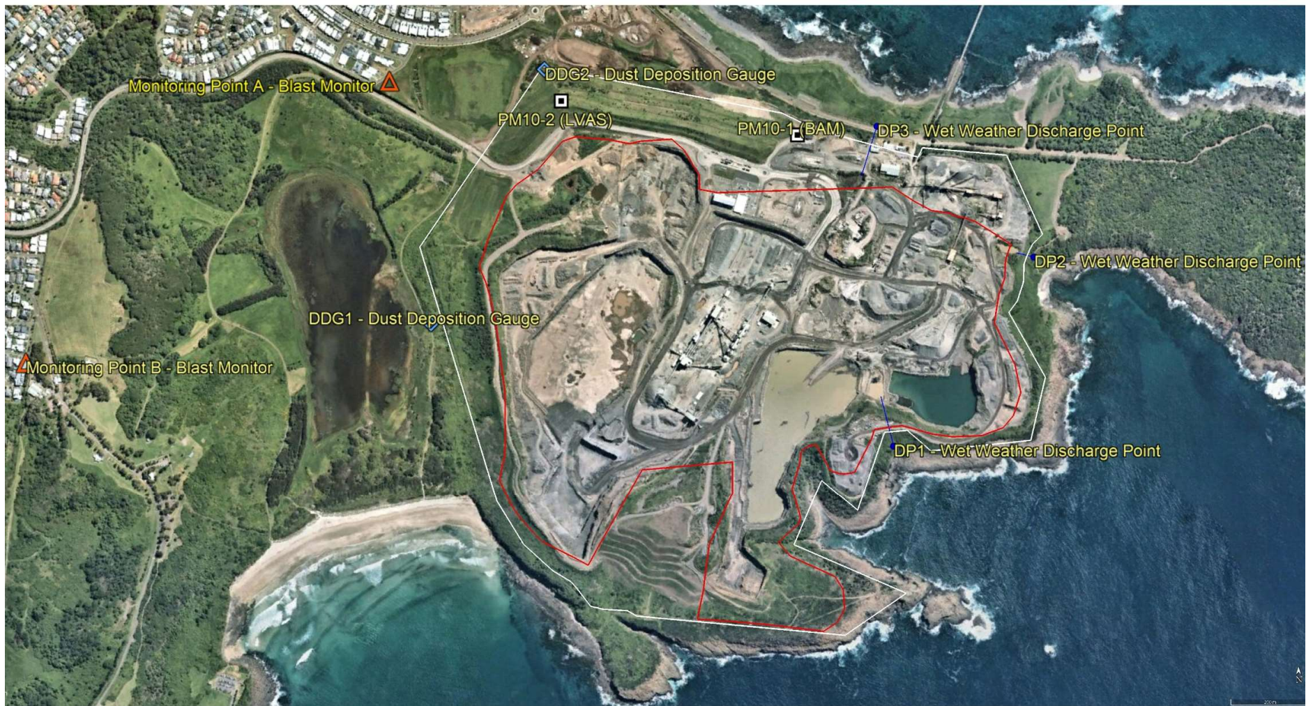
Figure 1: Monitoring locations at the Bass Point Quarry. Air quality monitoring locations have been acronymised as follows: DDG1 – Dust Deposition Gauge 1; DDG2 – Dust Deposition Gauge 2; PM10-1 – Continuous PM 10 Monitor; PM10-2 – Low Volume PM 10 Sampler.
