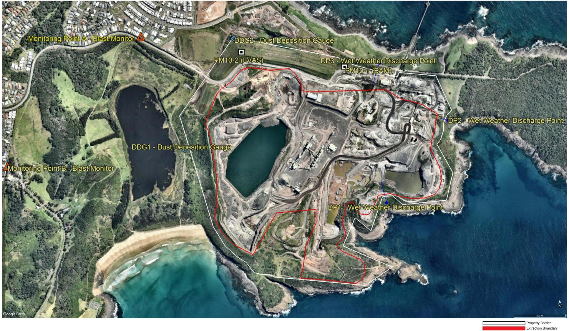
Figure 1: Monitoring locations at the Bass Point Quarry. Air quality monitoring locations have been acronymised as follows: DDG1 – Dust Deposition Gauge 1; DDG2 – Dust Deposition Gauge 2; PM10-1 – Continuous PM 10 Monitor; PM10-2 – Low Volume PM 10 Sampler.
