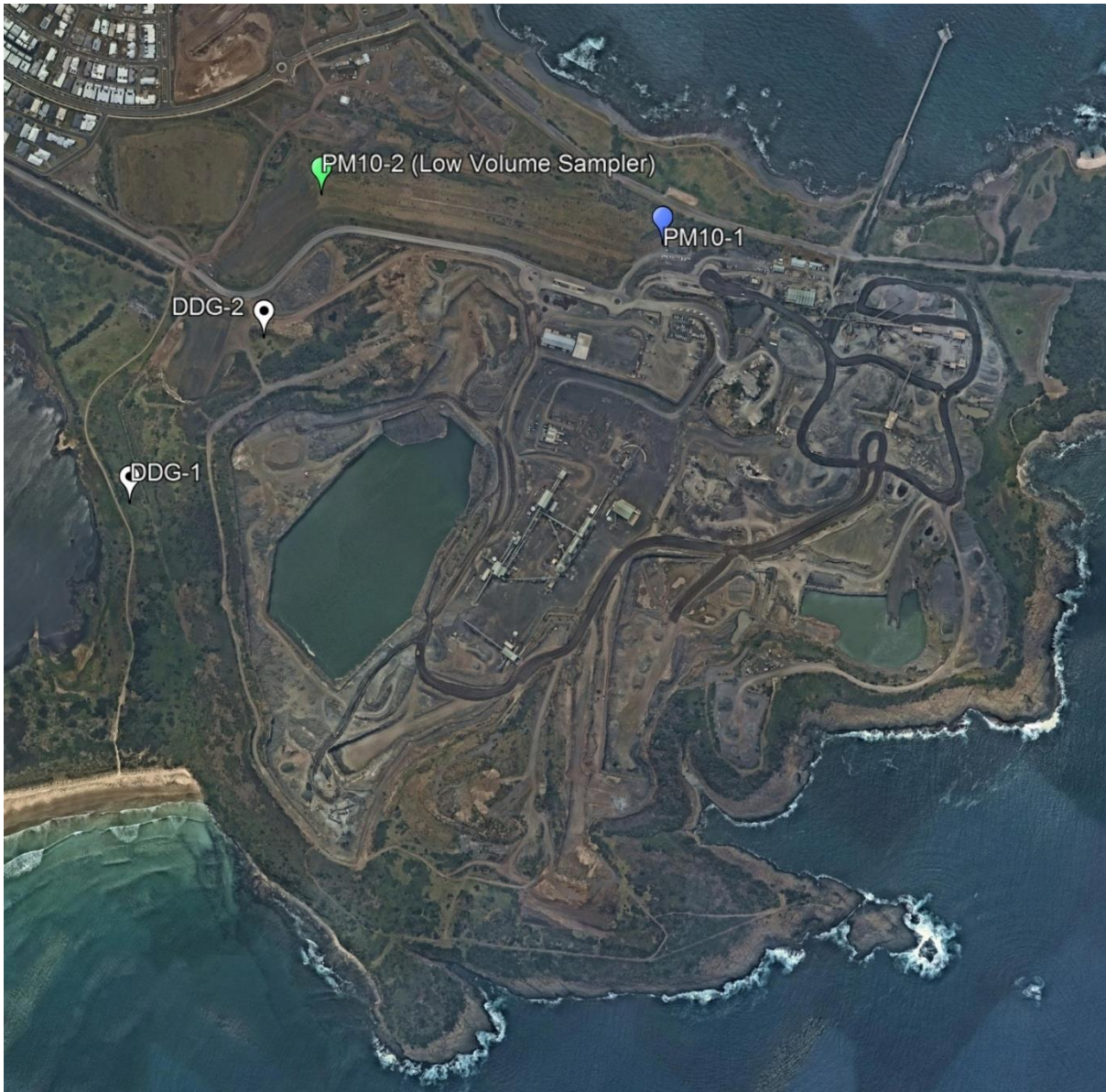
Figure 1: Air quality monitoring locations at the Bass Point Quarry. Locations have been acronymised as follows: DDG-1 – Dust Deposition Gauge 1; DDG-2 – Dust Deposition Gauge 2; PM10-1 – Continuous PM 10 Monitor; PM10-2 – Low Volume PM 10 Sampler.
