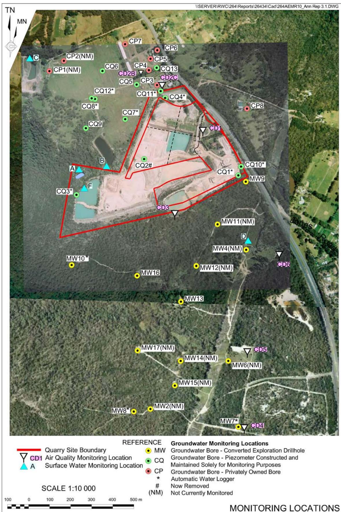
**Figure 1:** Rocla Calga Quarry environmental monitoring locations
