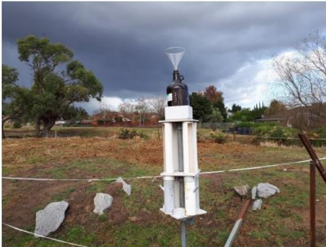
Directional Dust Deposition Gauge near Montague Cres.
