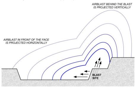
The airblast and noise emission in front of a blast face than greater than behind the face.
