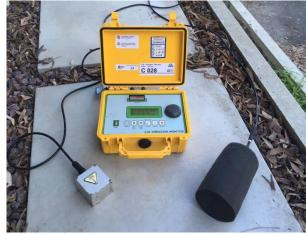
The blast vibration results are detailed in a compliance report which is sent to the quarry after each blast event and forwarded to the relevant authority.
